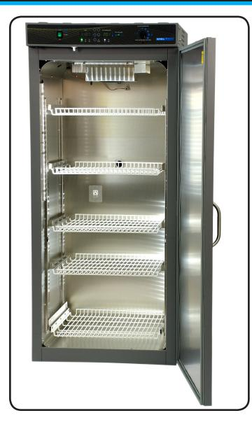
Expanding on our current thermoelectric (Peltier) refrigerated incubators, the SHEL LAB Drosophila units utilize day/night controls along with LED lighting to provide an excellent environment for drosophila culture. The cabinets are designed with a mechanical convection system to ensure a gentle and even air distribution. A programmable day/night microprocessor temperature controller and over temperature limit control ensure a proper and safe environment.
